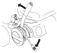
2 Remove the front hood by removing the pin.
